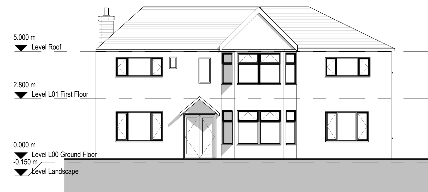
Existing South Elevation 1 : 100
